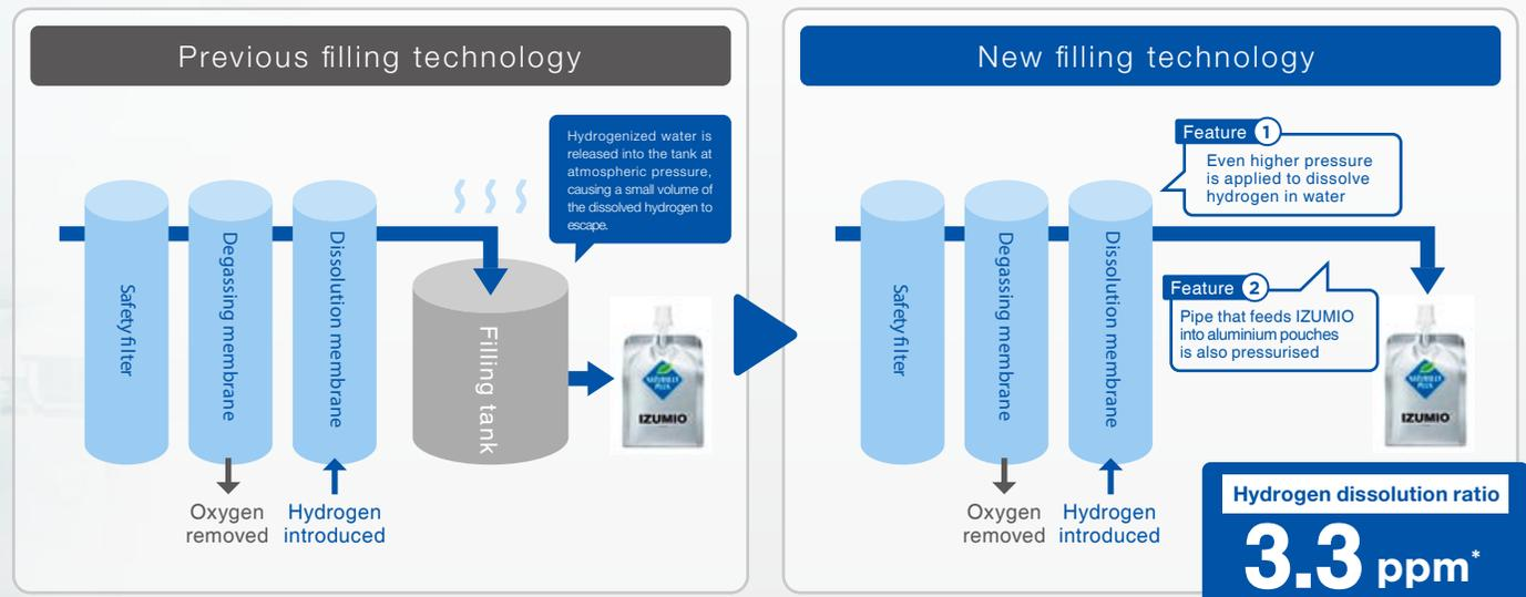
\* Average reading at point of filling, i.e. the point in the manufacturing process when the IZUMIO aluminium pouches are being filled.
